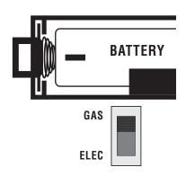
[DOWN = ELEC/HP] This setting runs the system's blower fan when heat is called for, and is required for heating systems that do not control their own fan while the thermostat is in HEAT mode. Heat pump systems, and units with an electric heating element typically require this setting.
